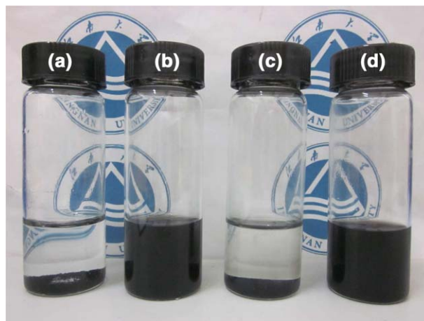
Figure 7. Water dispersions of MWCNTs (a) without dispersants (b) with \alpha -CD-C, and of SWCNTs (c) without dispersants (d) with \alpha -CD-C. The images were taken after one month storage. [Color figure can be viewed in the online issue, which is available at wileyonlinelibrary.com .]
